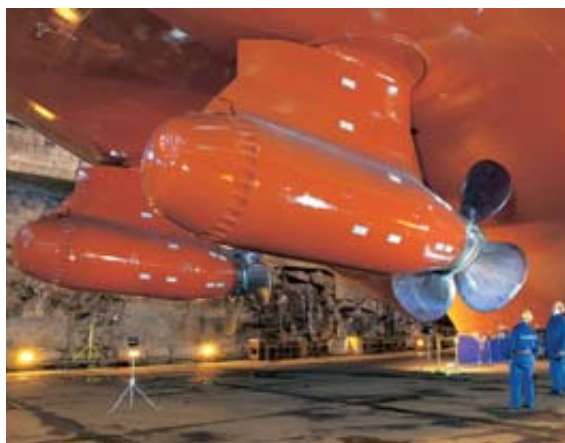
▼ Azipod® propulsion unit
