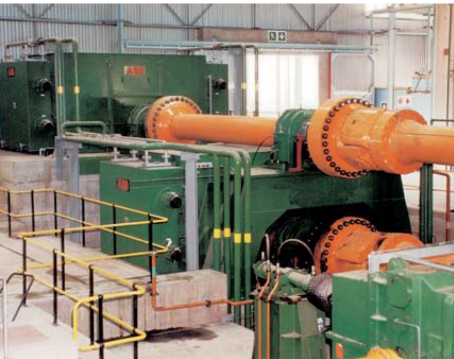
◀ Rolling mill motor (twin drive)
