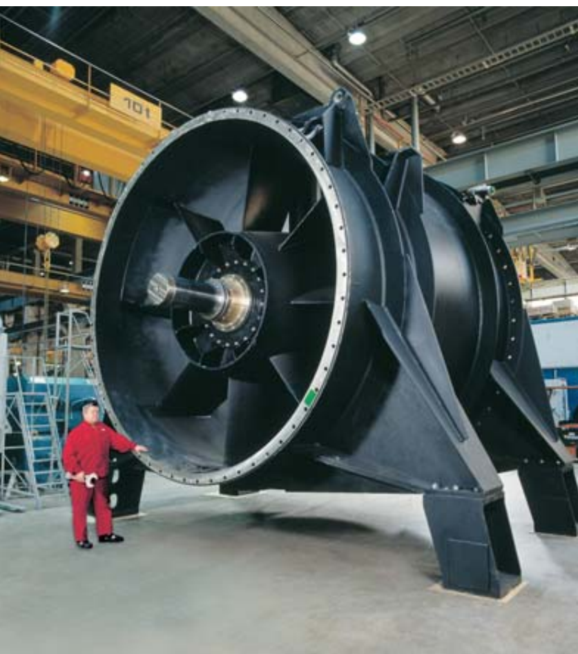
◀ Integrated submersible permanent magnet pump motor
